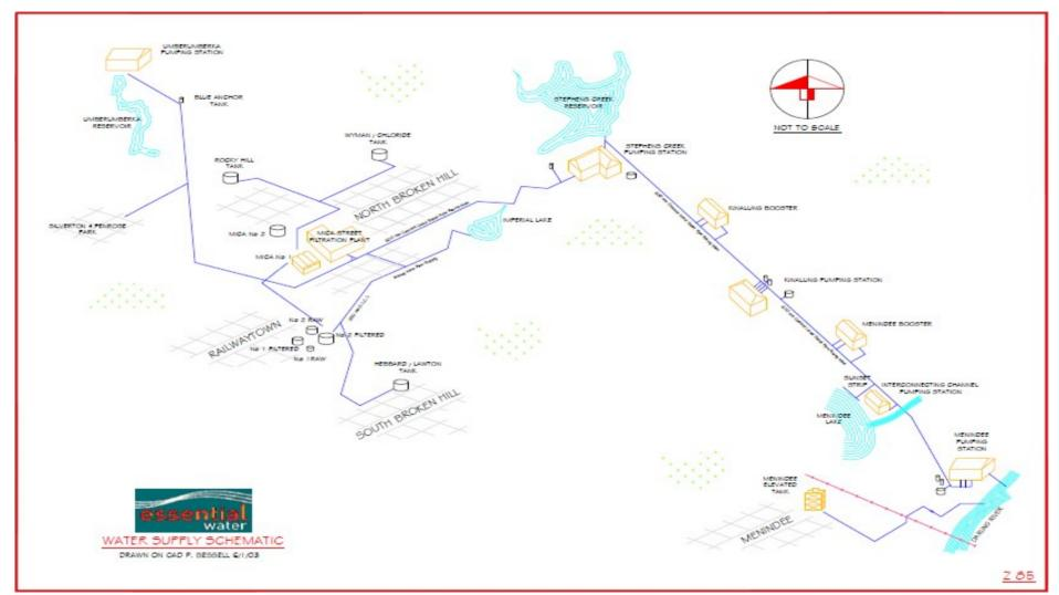
5.1 Attachment 1: Broken Hill Water Reticulation Schematic
